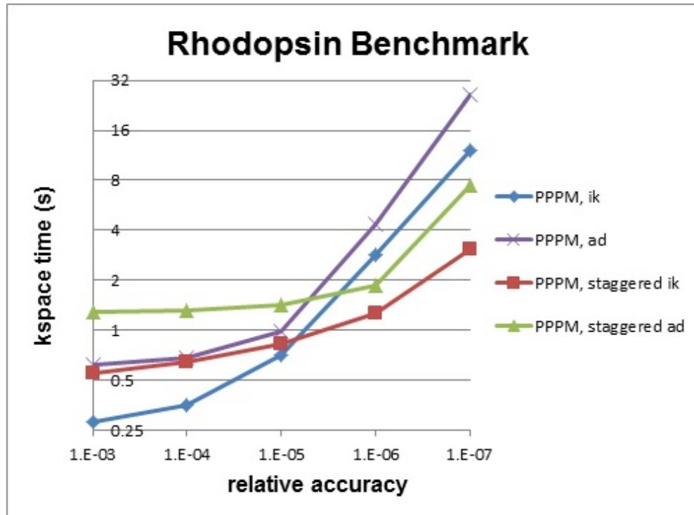
**IMPORTANT NOTE:** Using staggered PPPM may not give the same increase in accuracy of energy and pressure as it does in forces, so some caution must be used if energy and/or pressure are quantities of interest, such as when using a barostat.
