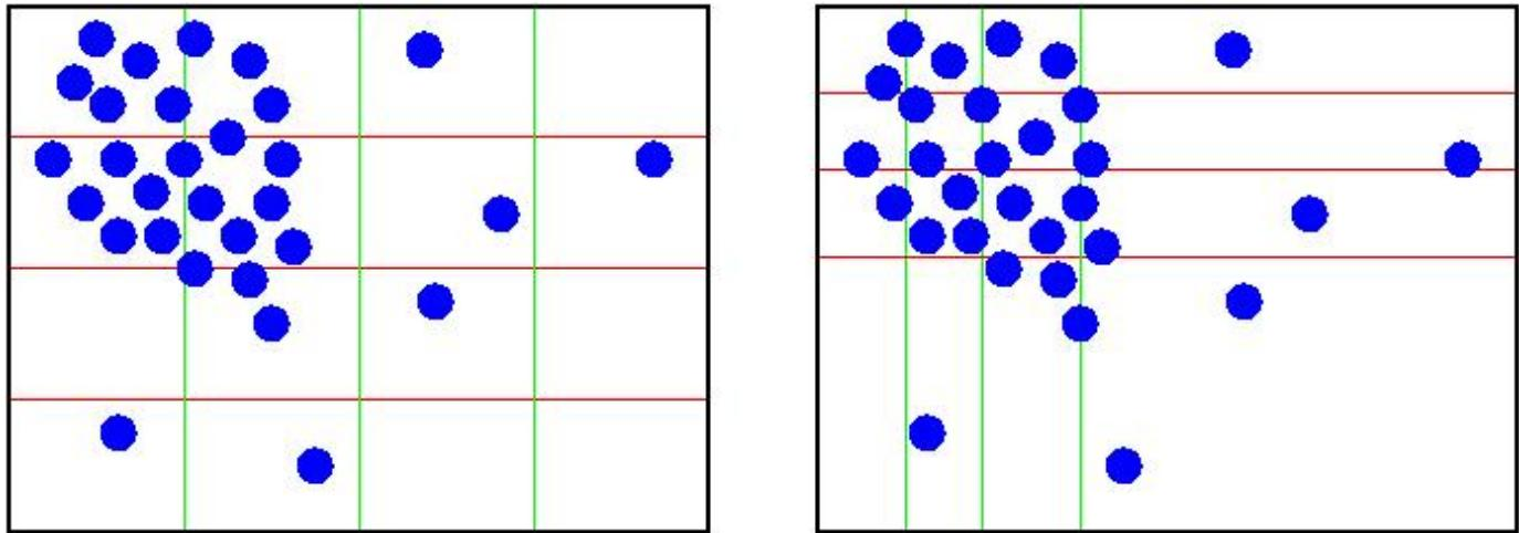
The *rcb* style is a "tiling" method which does not produce a logical 3d grid of processors. Rather it tiles the simulation domain with rectangular sub-boxes of varying size and shape in an irregular fashion so as to have equal numbers of particles in each sub-box, as in the following 2d diagram. Again the left diagram is the default partitioning of the simulation box across processors (one sub-box for each of 16 processors); the right diagram is after balancing.
