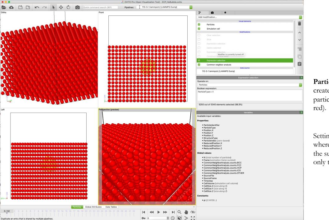
**ParticleType** is used to create a selection of particles (now colored in red).
