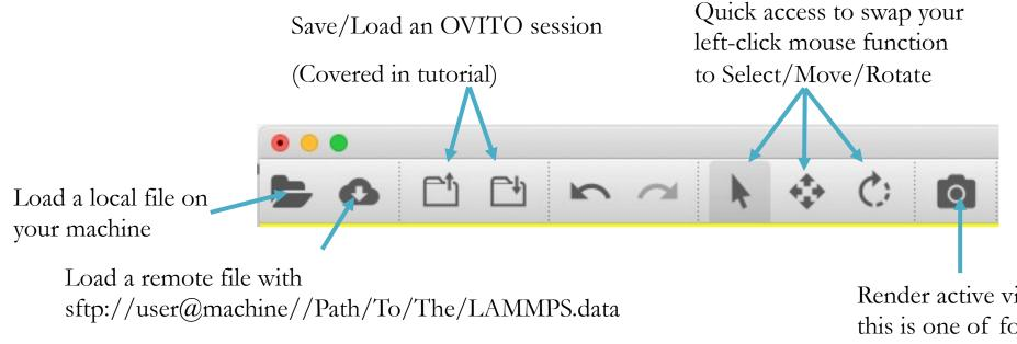
Very useful because OVITO deletes the temporary file when the app is closed, saving you a ton of disk space. Render active viewport, this is one of four panels highlighted in yellow
